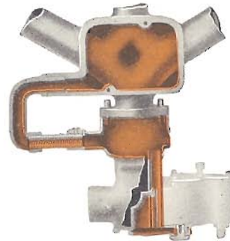
Sectional view of entire progressive heating system. Color shows areas in which heated exhaust gases circulate around intake manifold at top, carburetor throttle, and low speed throat, exhausting at bottom.
